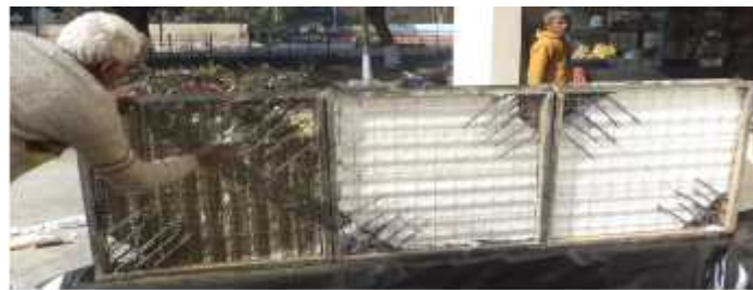
Figure 3.16 Preparation and application of cement slurry on specimen
