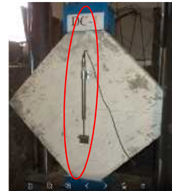
Figure 3.24 Cracking of specimen during diagonal compression test
