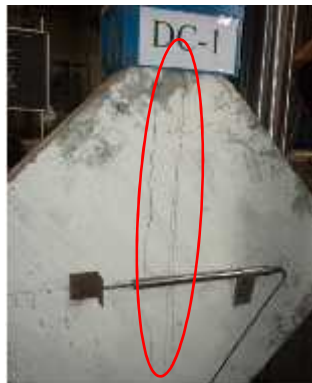
Figure 3.24 Cracking of specimen during diagonal compression test
