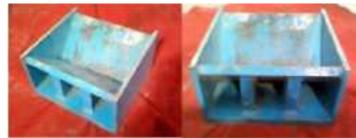
Figure 3.21 Test setup for diagonal compression test
