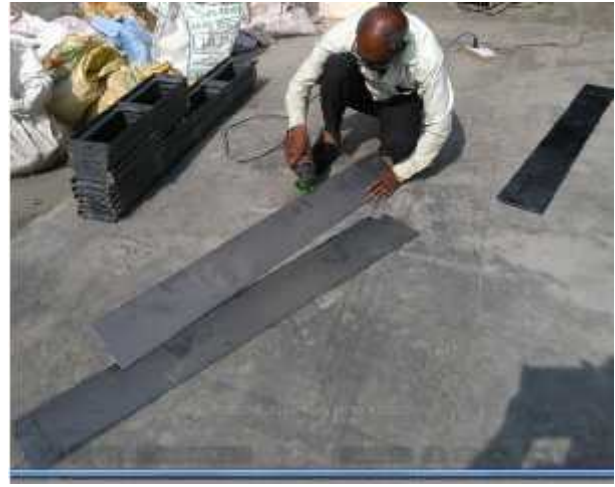
Figure 3.44 Fabrication of form for casting of flexural test specimen
