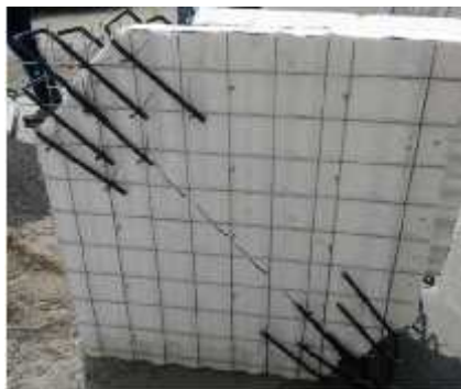
Figure 3.12 EPS panel with U-bars reinforcement in corners
