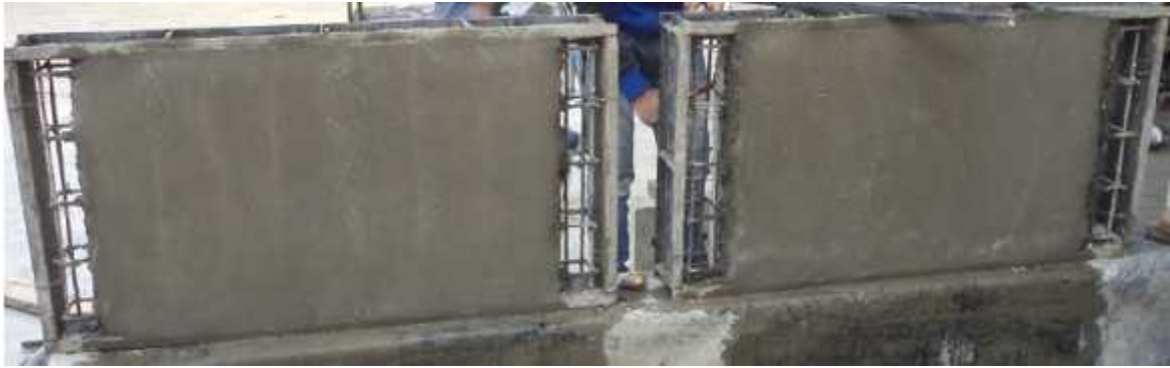
Figure 3.49 Construction of EPS panel for flexural test
