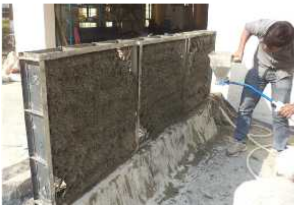
Figure 3.17 Application of concrete on face of specimen through spray
