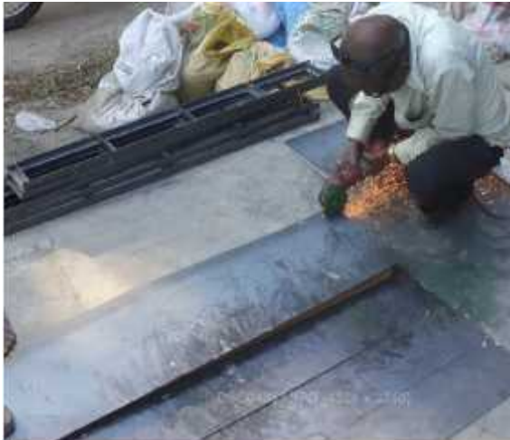
Figure 3.44 Fabrication of form for casting of flexural test specimen
