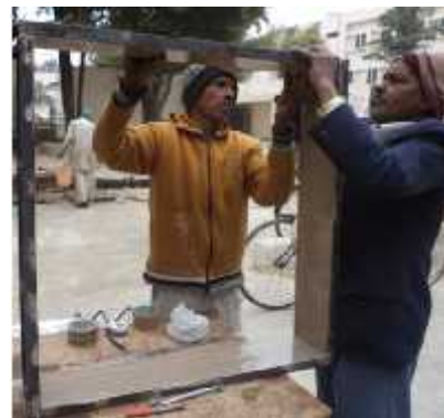
Figure 3.13 Assembling of casting frame
