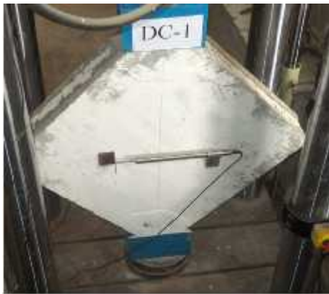
Figure 3.21 Test setup for diagonal compression test
