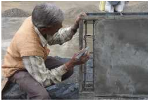
Figure 3.49 Construction of EPS panel for flexural test
