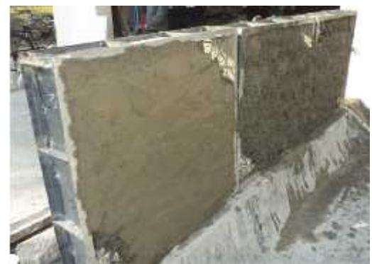
Figure 3.17 Application of concrete on face of specimen through spray
