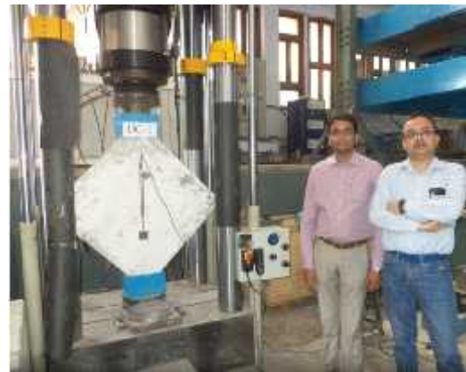
Figure 3.21 Test setup for diagonal compression test
